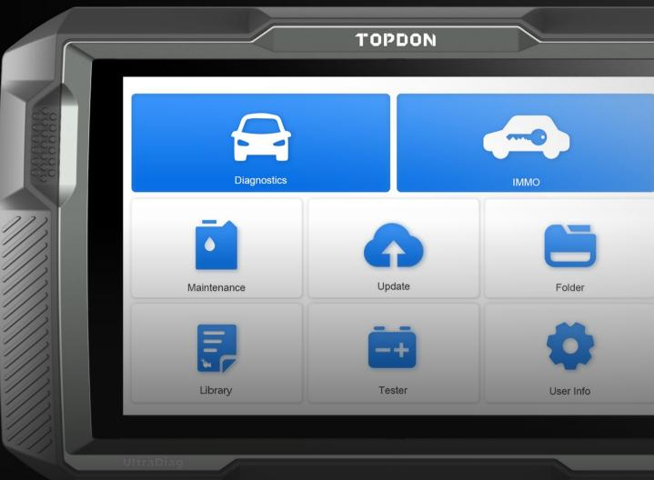
OS: Android 11.0 Storage Capacity: RAM 2G & ROM 32G Screen: 8 inches, 1280\*800 Resolution Connectivity: Bluetooth 5.0/SPP USB Wi-Fi
